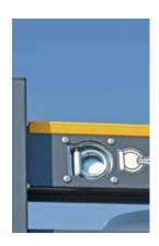
Load securing rings on the cab guard.
