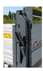
Gate posts with anti-vibration system (removable at the rear).
